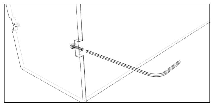
Tighten the screw gently with the 1.5mm hex key, do the same with the second screw on the same side,
