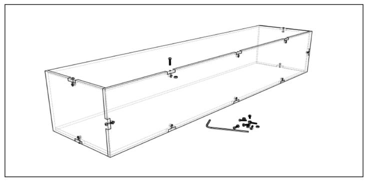
Slide the nut to one of the slots of the T-joints, place the screw from the top and tighten it gently.
