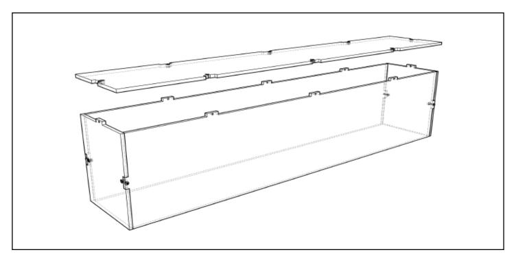
Place the top panel, and turn the box to one of its sides.
