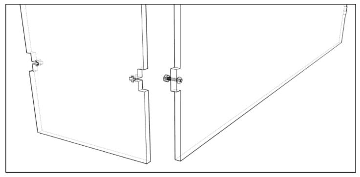
Insert one screw to one of the long side panel holes adjacent to the short side.
