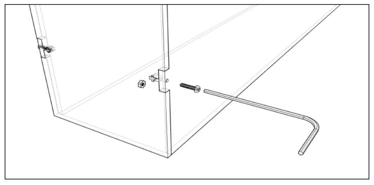
Alternatively, join the sides without screws, slide the screw nut into the slot, and place the screw through the hole into its screw nut.
