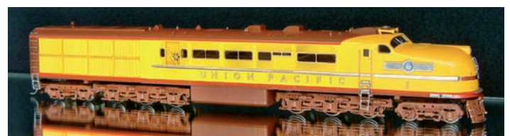
UP # 1 Steam Turbine Electric (4-6-6-4)
