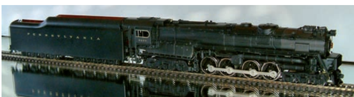
Pennsy S-2 Steam Turbine (6-8-6)
